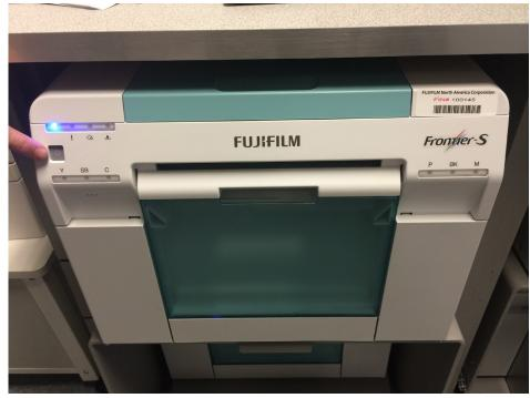
When the new printer is completely charged with ink you will see a solid blue light and a solid amber light above the paper.
