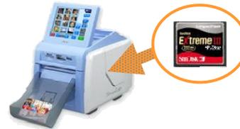
Insert the expansion CompactFlash card into the designated CompactFlash slot on the UP-CR10L.
