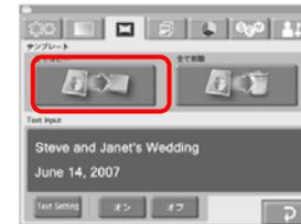
Copy the data from the memory card to the expansion CompactFlash card, using the template tab of the administration screen.
