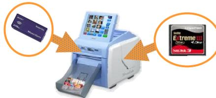
Insert the memory card and expansion CompactFlash card into the UP-CR10L.
